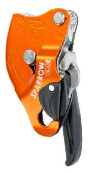
Self-braking descender for rope work has been developed for high workloads. It allows the operator to lower themselves on the working line, to position themselves on the working line and to ascend the same rope. It is ideal in the event of assisted lowering of two people with the device installed at the anchor (the operator lowers the rescuer and the person being rescued) or for simultaneous lowering of two people (rescuer lowers themselves with the injured person).
